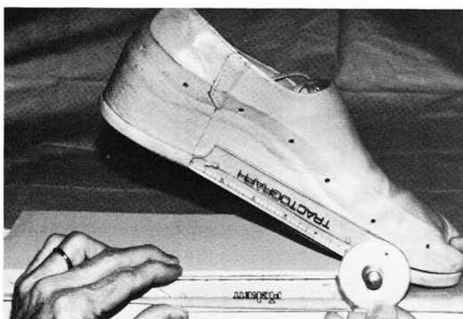
Fig. 1 C. Angle of decreased dorsiflexion requirement is measured with tractograph.
