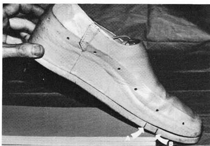
Fig. 1 B. Placement of 3/4 inch rocker under sulcus of proximal phalanx.
