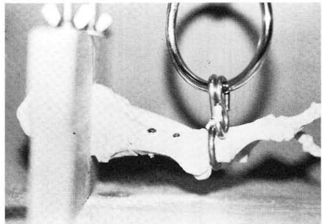
Fig. 4. Experimental model designed to quantify relative stress/strain properties in first metatarsal osteotomies. The midfoot is rigidly secured while dorsal forces are applied to the first metatarsal-phalangeal joint.
