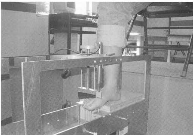
Figure 1. First ray dorsal mobility assessment device used in this study.
