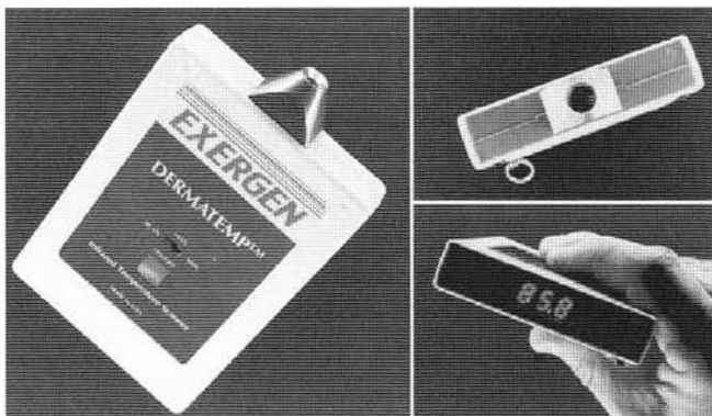
Figure 2. Exergen Dermatemp hand-held scanner – arrows point to sensing lens, 4 mm diameter. Momentary depression of scan button (red button) will provide instantaneous temperature readings in a tenth of a degree, Celsius or Fahrenheit.
