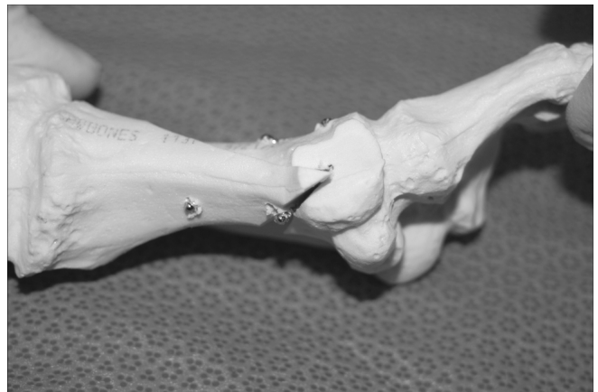
Figure 4. Loading of bone model illustrating slippage of the plantar arm of the osteotomy.
