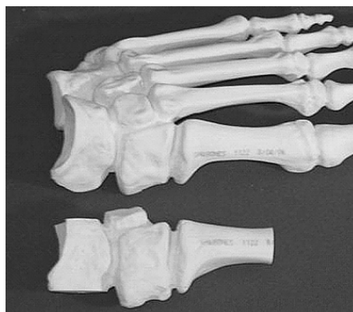
Figure 1. Sawbones specimen prepared for testing.
