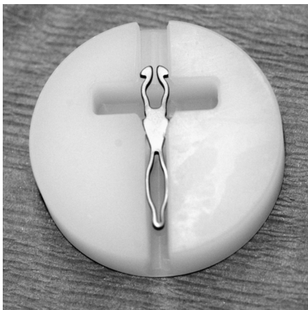
Figure 1. Smart Toe implant in its contracted state.
