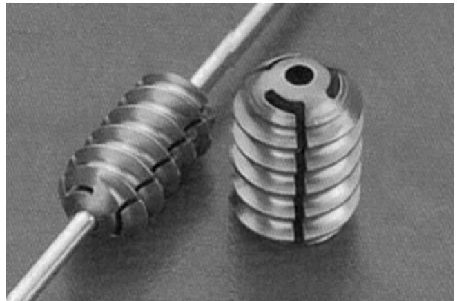
Figure 5. Maxwell-Brancheau Arthroereisis (MBA) Implant. This was the first arthroereisis implant fabricated (by Kinetikos Medical, Inc, Carlsbad, CA) completely of metal (titanium). It is cannulated and threaded with unique slots incorporated into the design for tissue ingrowth.
