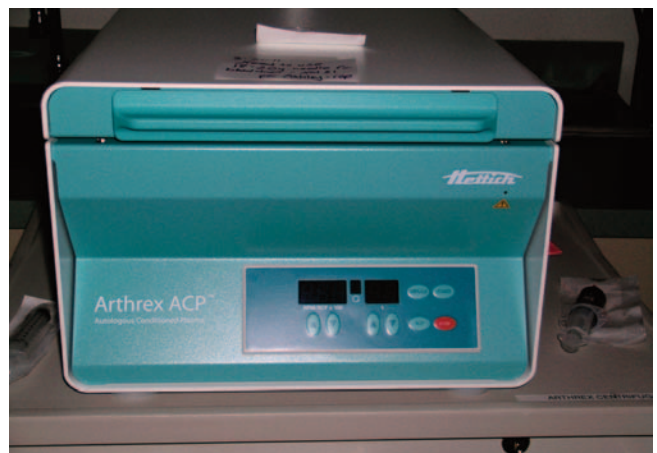
Figure 6. The bench top centrifuge is run at 1500 rpm for 5 minutes.
