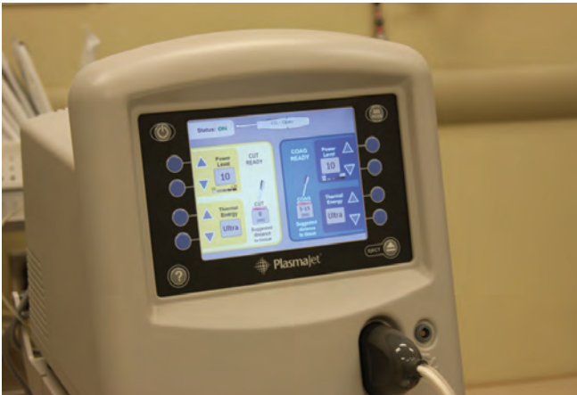
Figure 3. PlasmaJet settings are simplified as yellow (cutting) and blue (coagulation) for consistency with existing hand-held coagulation modules. Power level and thermal energy are adjustable, and the program directs the user on suggested distance from the target tissue for optimal effect. Depicted is the lowest setting of the range available, which is suggested for initiation of cutting to determine tissue response.
