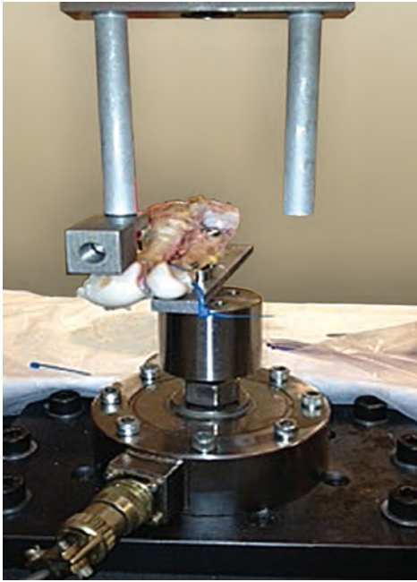
Figure 2. Specimen fixated to Instron 8511, second metatarsal fixated to a custom plate and first metatarsal being loaded from plantar to dorsal recreating ground reactive forces.
