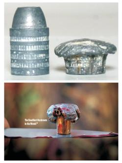
Figure 6. Comparatives of flattening between lead conical bullet and a lead bullet surrounded by a brass jacket.
