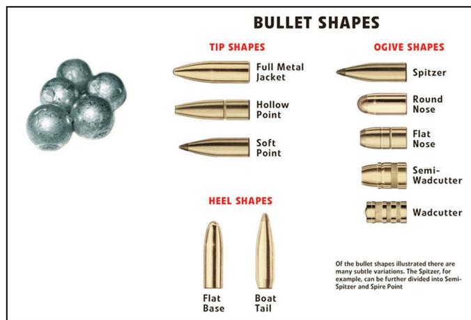
Figure 1. Examples of projectiles ranging from lead musket balls to modern bullet shapes.
