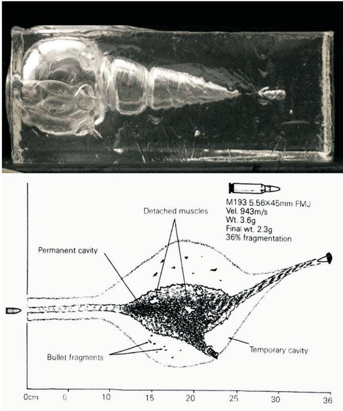
Figure 12. Examples of shock waves that follow high velocity projectiles in ballistic gel and the tendency for small weight projectiles to fragment and tumble.
