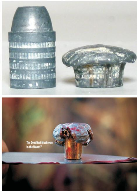
Figure 6. Comparatives of flattening between lead conical bullet and a lead bullet surrounded by a brass jacket.
