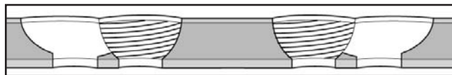
Figure 1B. Locking plates allow a screw to engage and lock into the threaded portion of the plate.
