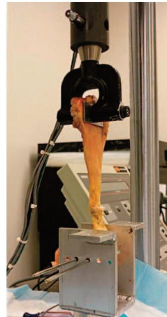
Figure 4. A Steinmann pin was placed transversely through the calcaneus and secured to an adapted load cell portion of the Instron machine.
