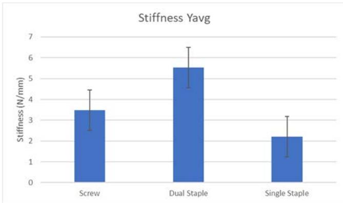
Figure 4: Representation of stiffness of fixation methods for first metatarsal closing base wedge osteotomy.
