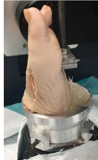
Figure 2. Picture of specimen mounted to Vivo test machine (AMTI).
